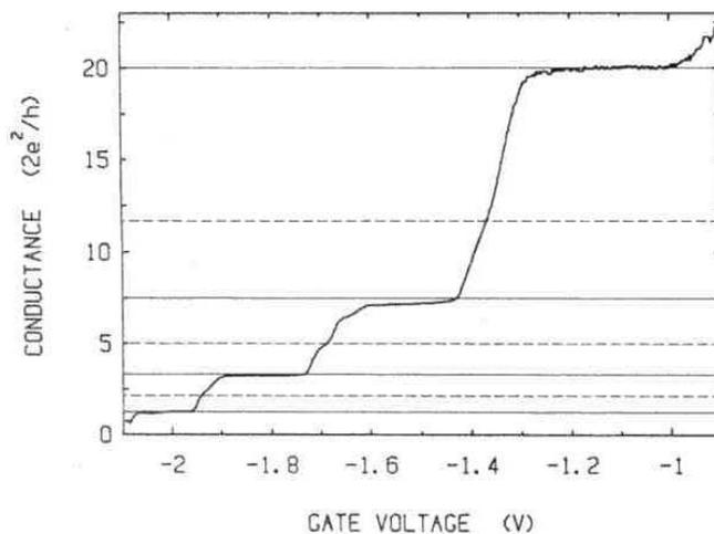
Figure 5: Longitudinal conductance  $G_L$  as a function of voltage on the point-contact gate.
