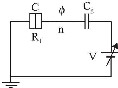
Figure 8: Schematic of the single electron box
