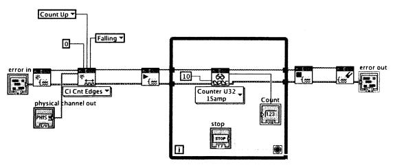
a) The Block diagram of a VI to read a counter using DAQmx is shown above. The first DAQmx VI to be executed defines a new DAQmx task.
