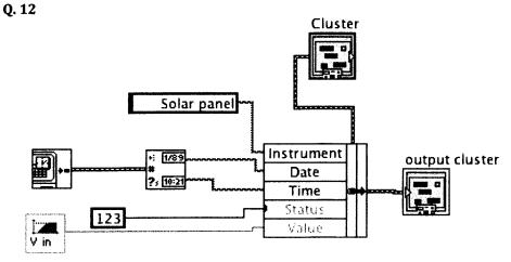
The block diagram above shows where data, about a solar energy system is bundled into a cluster.
