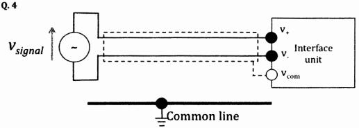
a) The circuit above shows represents a single-ended voltage measurement.
