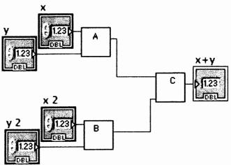
a) In the block diagram above C executes as soon as A or B has finished execution.
