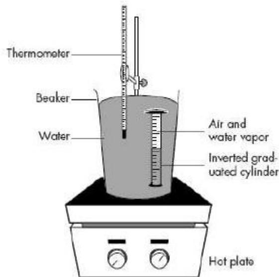
Figure 1: *The measuring equipment for determining the absolute zero.*
