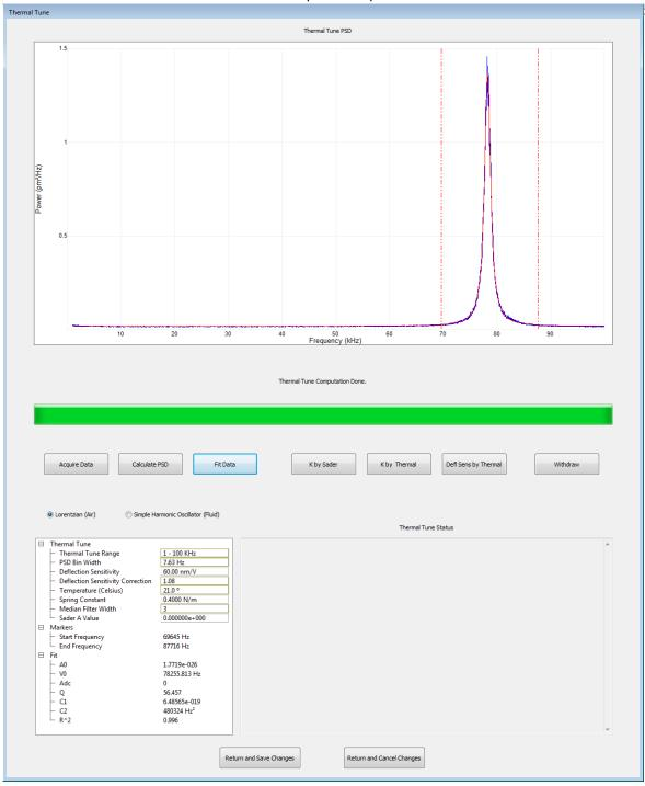
5. You can press K by Thermal and Defl Sens by Thermal to get initial values for them. Make a note of the resonant frequency (V0), Quality factor (Q) and Spring constant. You will need these later.
