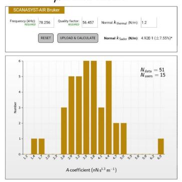
\* Error estimate (95% C.I.) for the spring constant,  $k_{\rm Sader}$ , is derived from the histogram.
