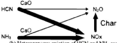
(b) Heterogeneous oxiation of HCN and NH<sub>3</sub> over CaO combined with NOx reduction by char
