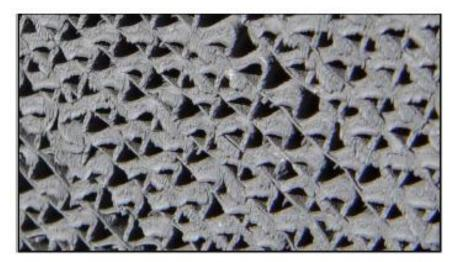
Silicate layers on a catalytic afterburner Source: Pierce (2005)
