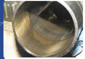
Gold-coloured siloxane layer on the inner surfaces of a cylinder Source: Environmental Agency (2002)
