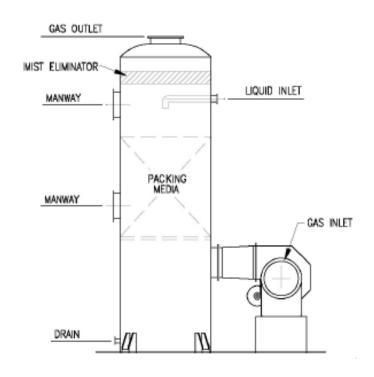
ammonia is stripped out from the digestate using the counter-current exhaust air from the CHP unit (some 80-90° C) and then recovering ammonium sulfate in the second step of the process.
