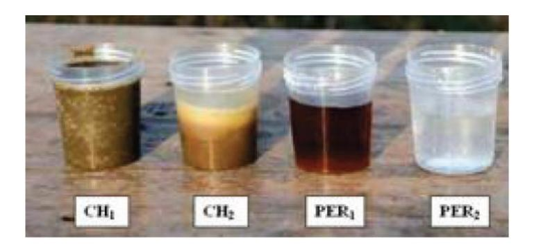
CH1: liquid effluent from the solid/liquid separation
