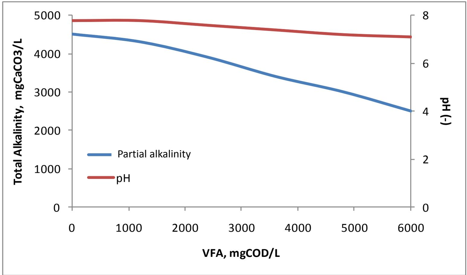
pH versus partial alkalinity for increasing VFA concentrations in the AD reactor
