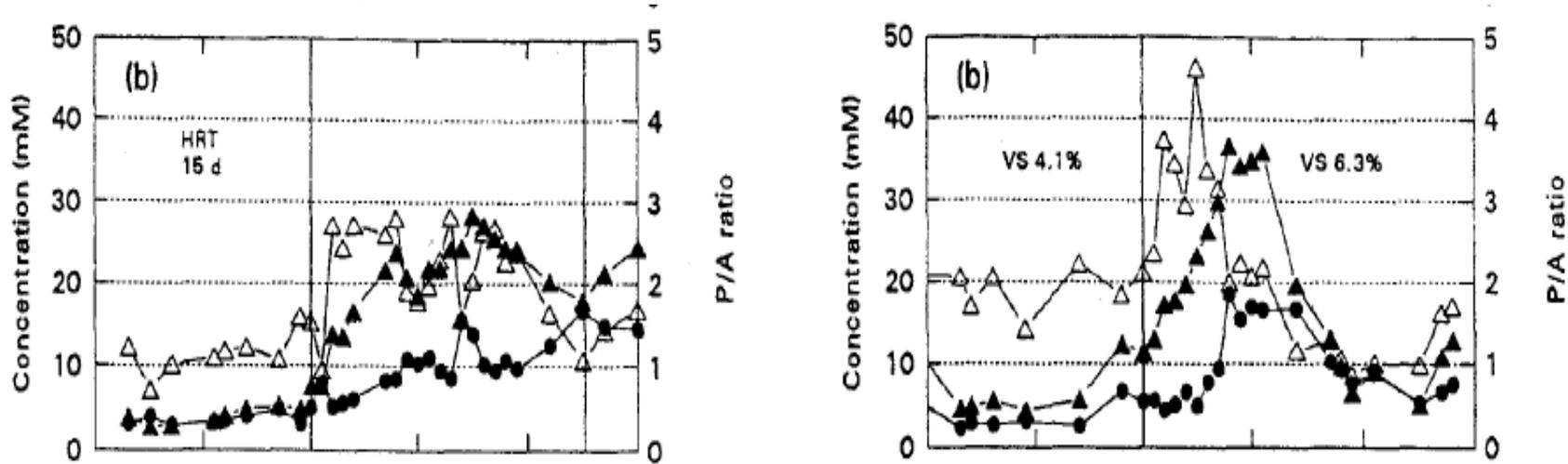
Changes in acetate ( $\Delta$ ) and propionate ( $\blacktriangle$ ) concentrations and P/A ratio ( $\bullet$ ) after a change in the HRT (left) and organic loading (right) (from Ahring et al., *Appl Microbiol Biotechnol* 43(1995), 559)
