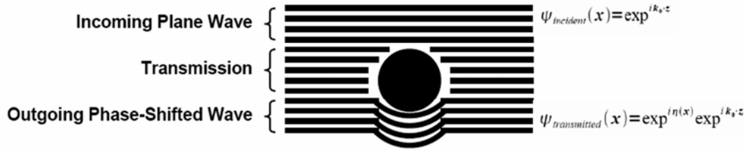
Figure 7.3. Schematic of the incoming and outgoing electron wave fronts during imaging. The incoming electrons can be approximated as a planar wave with constant phase. Upon interaction with the sample, the transmitted wave experiences a phase shift relative to its incoming phase, generating phase-based contrast.
