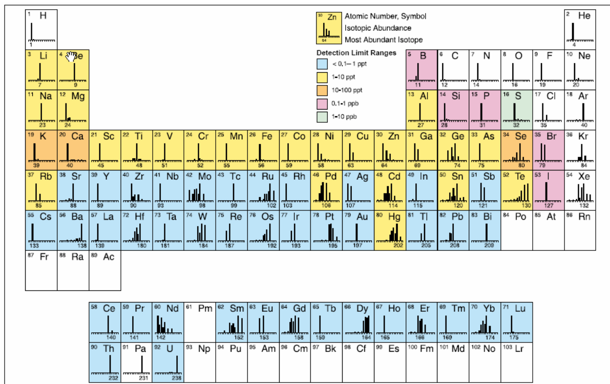
Figure 7. Approximate detection capabilities of the ELAN 6000/6100 quadrupole ICP-MS. (Courtesy of PerkinElmer, Inc.)
