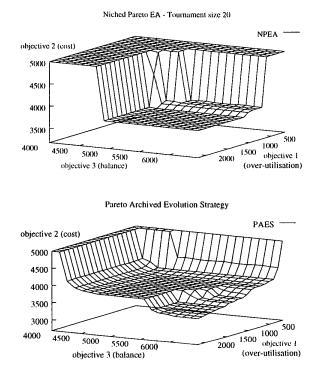
Figure 3: Nondominated surfaces obtained on an off-line routing task
