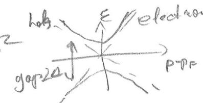
There are no quasiparticles with  $|\epsilon| < \Delta$ . This gap determines superconducting properties, because the electrons can flow without scattering.
